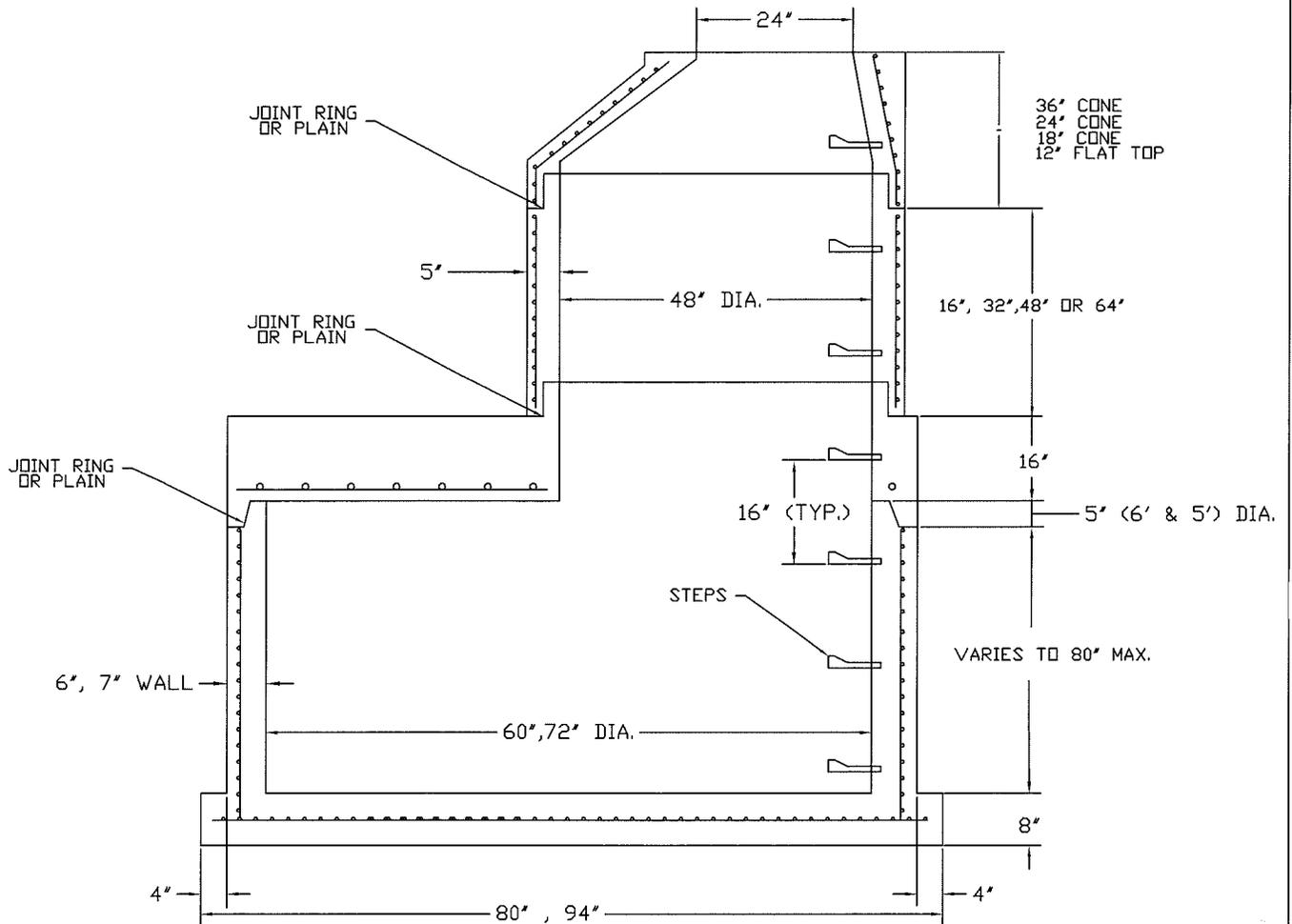
CONFORMS TO ASTM C-478
