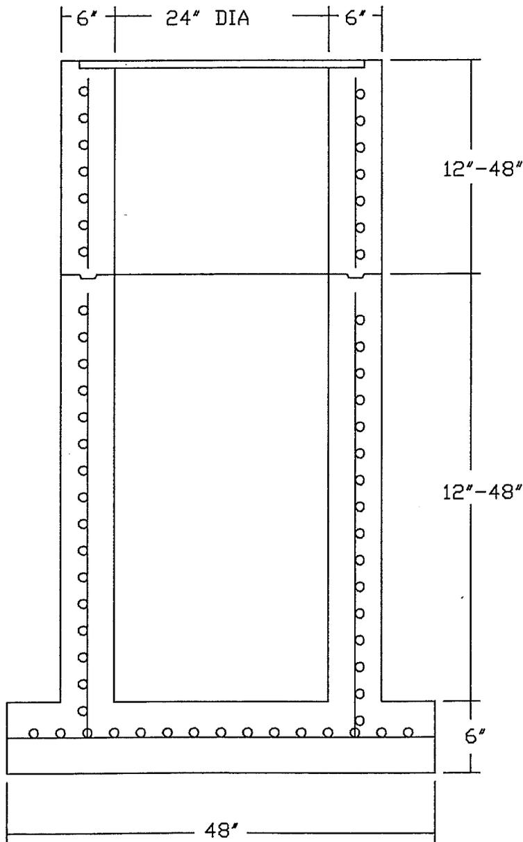
CONFORMS TO ASTM C-478
