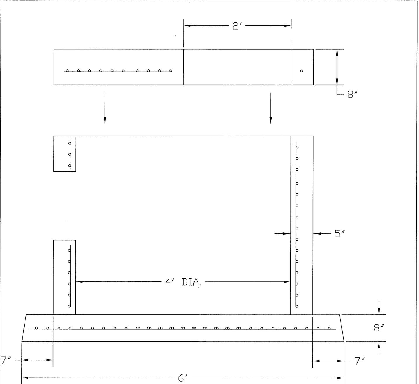
CONFORMS TO ASTM C-478
